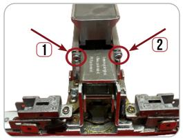
**3.** Slide off Housing to expose Pushpad & Baserail Assembly.
