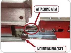
**9.** Slide Baserail motor side 1st back into the exit device Housing. Make sure the Motor & baserail go into the proper channels.
