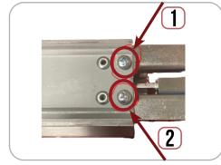
**10. Re-install (2) Screws** securing Housing to Baserail.
