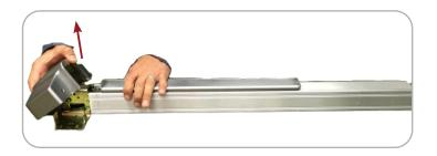
2. Remove (2) Screws securing Housing to Baserail.
